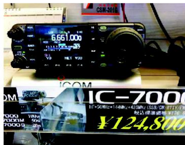
Fig 04: This Icom IC-7000 radio is set up for the Japanese VHF UHF bands. Note that the bands start at 144 and 430 MHz and may offer difficulty here in the USA. Look to the lower left and note also that this radio is offered in three versions of power output to provide for the license classes in Japan. It also is sold with a Japanese domestic warranty and I consider this version not attractive for purchase in Japan for use here in USA. It is also likely more expensive than offered by US Ham dealers.
