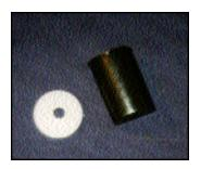
Begin by drilling a hole in the cover of the cassette container that is same diameter of the coax you are using.
